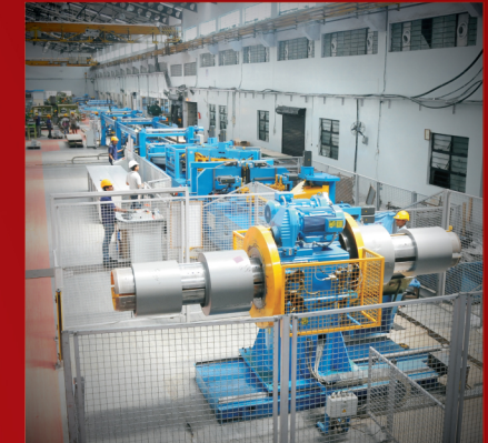
Automated Georg (German) CNC line for cutting and auto stacking
